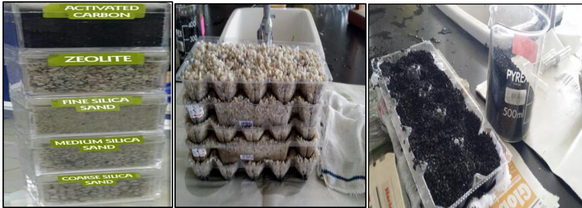
Figure 1: Assembly of the permeable system. From left to right: samples of the permeable materials used. Note that the order of the layers were inverted as conventional filtration systems pump upwards; layers of silica and zeolite arranged as upper and midsections of the system; activated carbon packed into the egg carton half forming the second last layer of the system.
