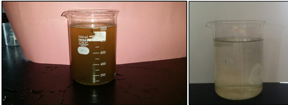
Figure 3: Filtration test results. From left to right: initially collected storm water; filtered storm water.
