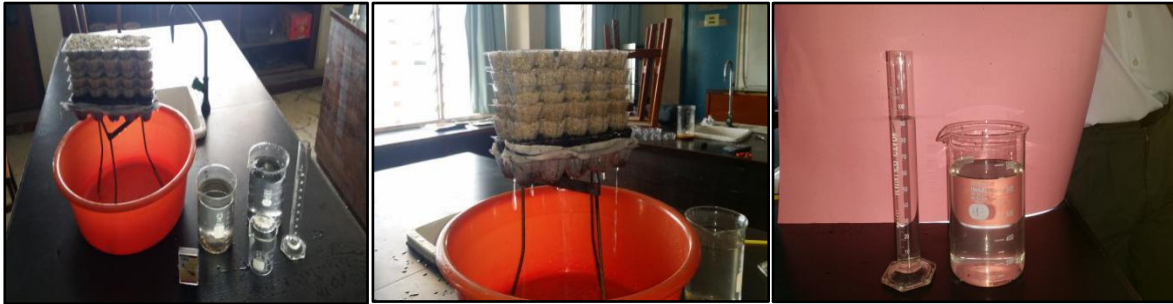
Figure 2: Testing infiltration of water. From left to right: Assembly of the general apparatus and system; infiltration of water through the permeable system subsequent to introduction; measuring the volume of effluent.
